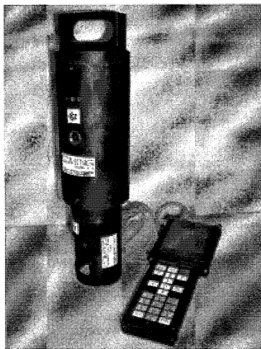
Fig. 12 COMTEST® OP 3/X pull-off apparatus provided with an accumulator motor for force generation.
